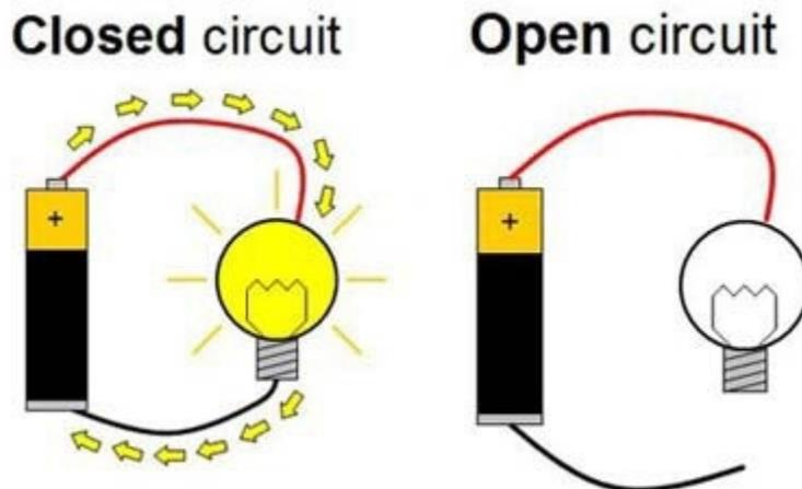
So what we want to do is create a CLOSED circuit where a battery serves to drive a motor that we will use to make a drawing robot!
